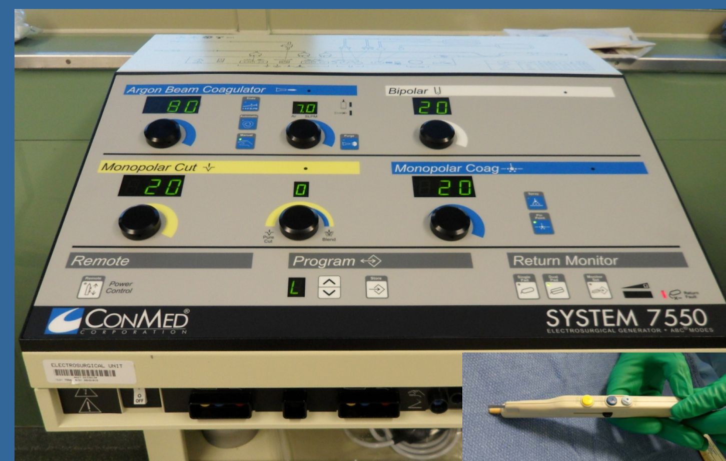
Figure 1. Argon beam coagulator ConMed System 7550 with its hand piece bottom right corner.
