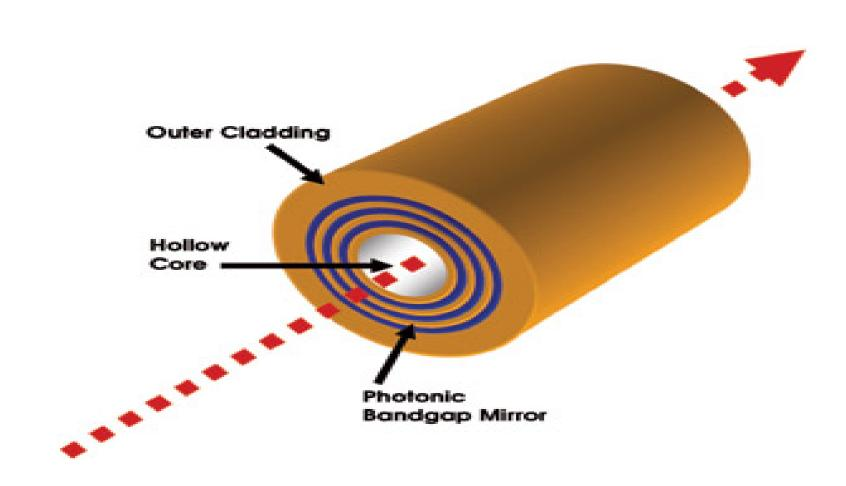
This allowed the CO2 laser beam to turn corners for the first time.CO2 has advantages over other flexible lasers (Thullium, Pulse-Dye-Laser and KTP) because its wavelength permits excellent haemostasis and sub-millimetre cutting precision with minimal surrounding thermal damage.
