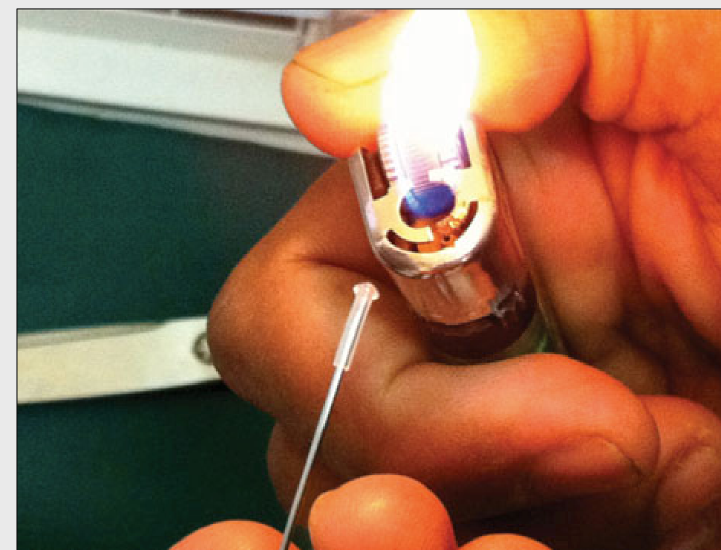
Figure 3. The lighter flame is used to partially melt and roll the free edge of the tube section..
