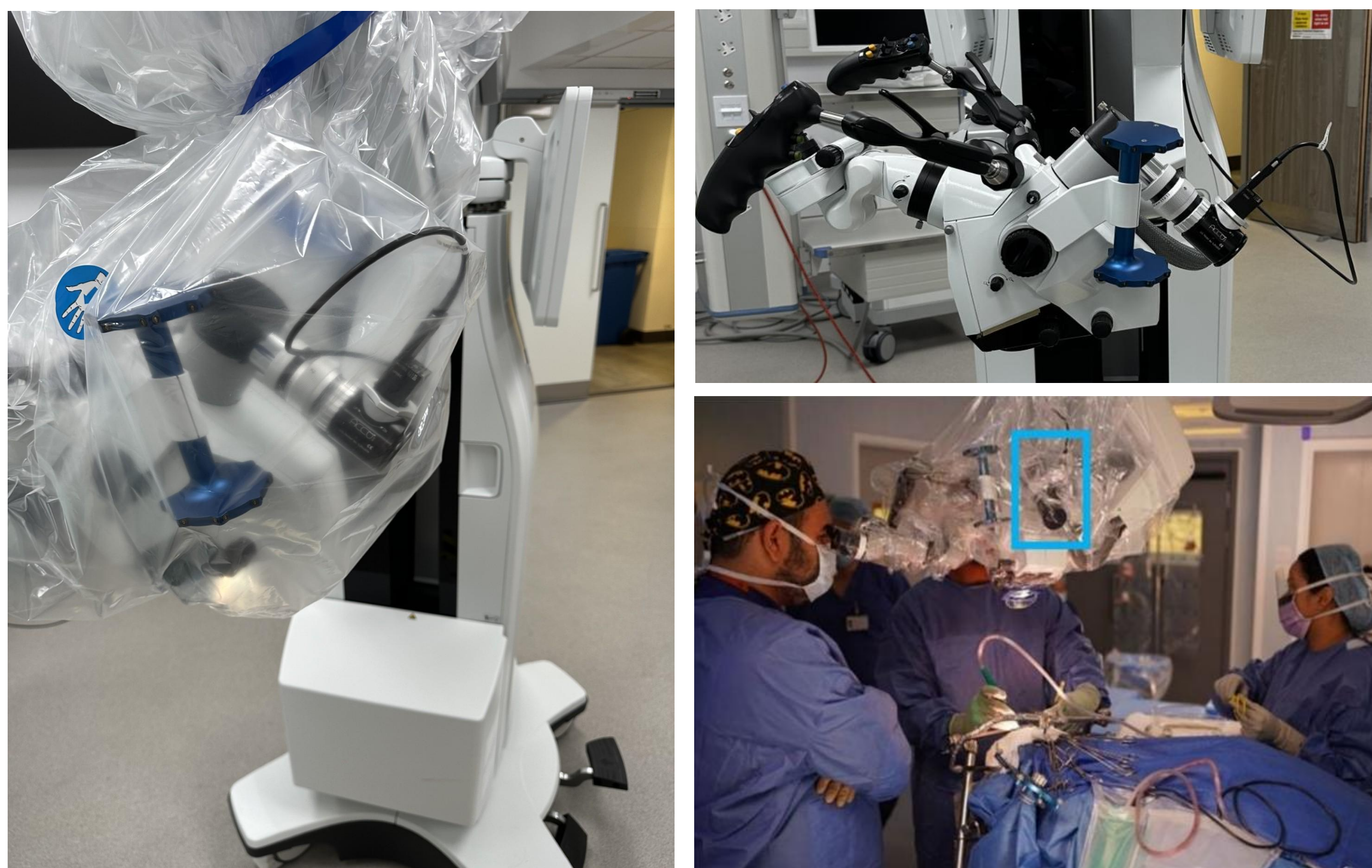
Figure 1. Snapshot mosaic hyperspectral camera mounted to Zeiss Kinevo-900 neurosurgical operating microscope
